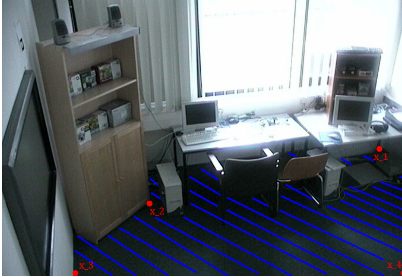
Figure 3.3: Our room with the 4 point correspondences x_1, \dots, x_4 (red), which embrace the ground plane of our room (blue).
