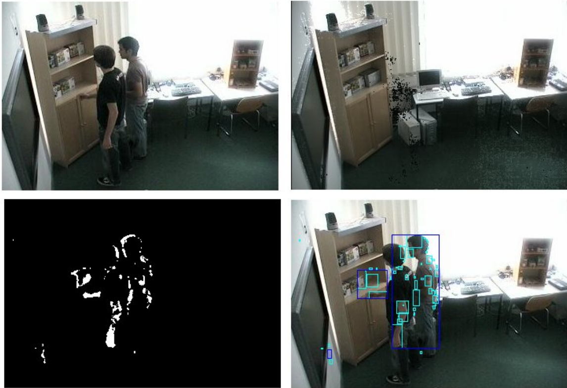
Figure 5.3: Top Left: Frame from one of the macro-tracking cameras. Persons are standing more or less static in front of the shelf. Top Right: Background model. Note the incorporation of the two persons into the model. Bottom Left: Result of background subtraction. Bottom Right: Result of region detection does not detect the two persons properly.
