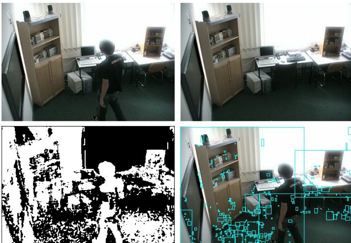
Figure 5.2: Top Left: Frame from one of the macro-tracking cameras. Person is walking across window. Top Right: Background model. Bottom Left: Result of background subtraction. Bottom Right: (Useless) result of region detection.
