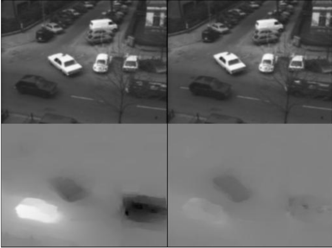
Figure 11.5: Computation of the optical flow for the taxi sequence (frames 15 and 19) with \alpha = 0.6 , s = 0.1 , \sigma_0 = 10 , \sigma_n = 0.8 , and \eta = 0.95 .
