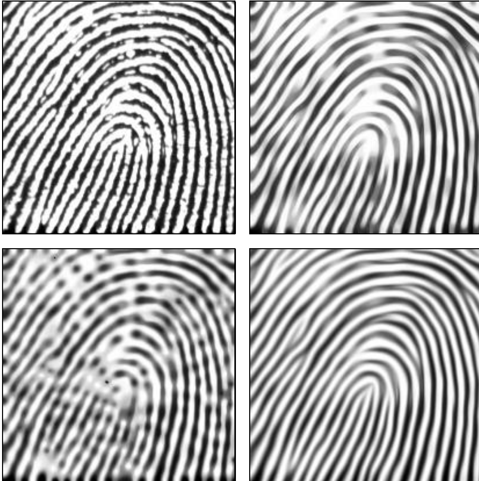
Figure 6.2: Anisotropic equations applied to the fingerprint image. (a) TOP LEFT: Original image. (b) TOP RIGHT: Mean curvature motion, t = 10 . (c) BOTTOM LEFT: Anisotropic diffusion similar to the Cotto-Germain model, \alpha = 0 , \sigma = 2 , t = 20 . (d) BOTTOM RIGHT: Coherence-enhancing anisotropic diffusion, \sigma = 0.5 , \rho = 4 , t = 20 .
