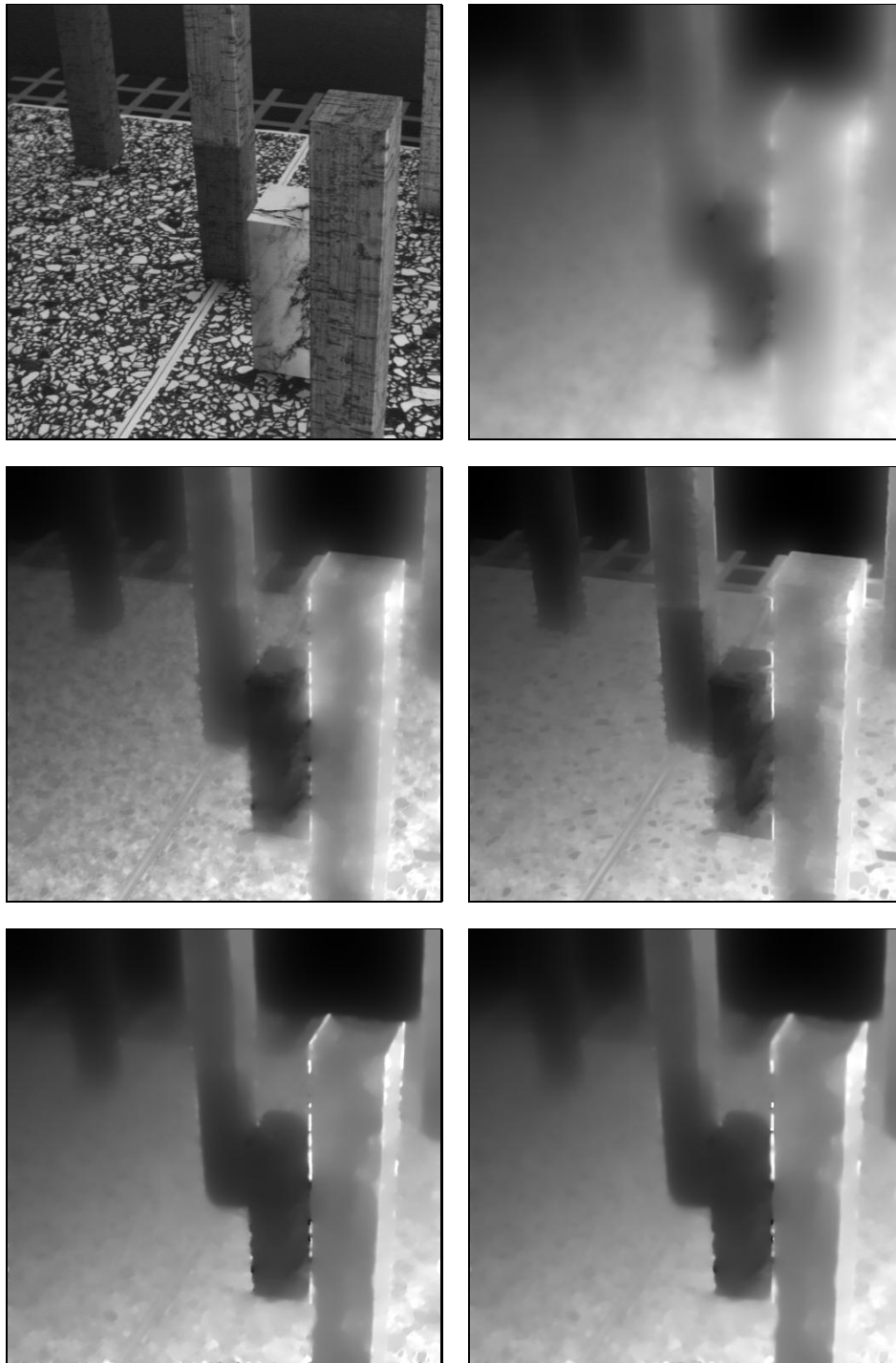
Figure 13.1: (a) TOP LEFT: Frame 16 of the marbled block sequence ( 512 \times 512 pixels). (b) TOP RIGHT: Optic flow magnitude between Frame 16 and 17 for homogeneous regularization. (c) MIDDLE LEFT: Result for image-driven isotropic regularization (d) MIDDLE RIGHT: Image-driven anisotropic regularization. (e) BOTTOM LEFT: Flow-driven isotropic regularization (f) BOTTOM RIGHT: Flow-driven anisotropic regularization.
