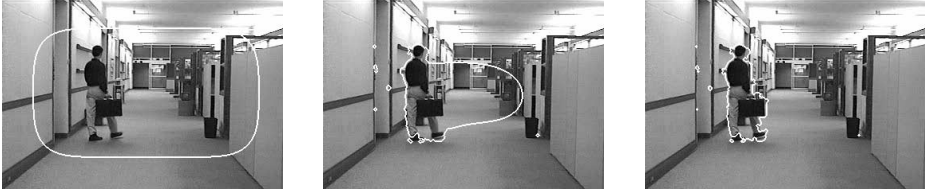
Fig. 2. AOS-based geodesic active contour model on hall-and-monitor image (size 352 \times 240 , \tau = 5.0 , k = -0.02 , \sigma = 0.5 , \lambda = 1 ). From left to right: 100, 500, 1000 iterations.
