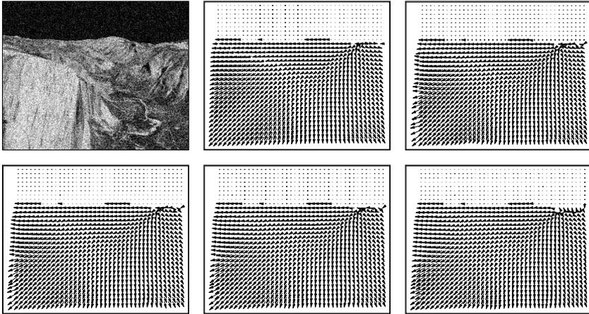
**Fig. 1.** (a) *Top left:* Frame 8 of the Yosemite sequence severely degraded by Gaussian noise with  $\sigma_n = 40$ . (b) *Top middle:* Ground truth flow field. (c) *Top right:* Computed flow field for  $\sigma_n = 0$ . (d) *Bottom left:* Ditto for  $\sigma_n = 10$ . (e) *Bottom middle:*  $\sigma_n = 20$ . (f) *Bottom right:*  $\sigma_n = 40$ .
