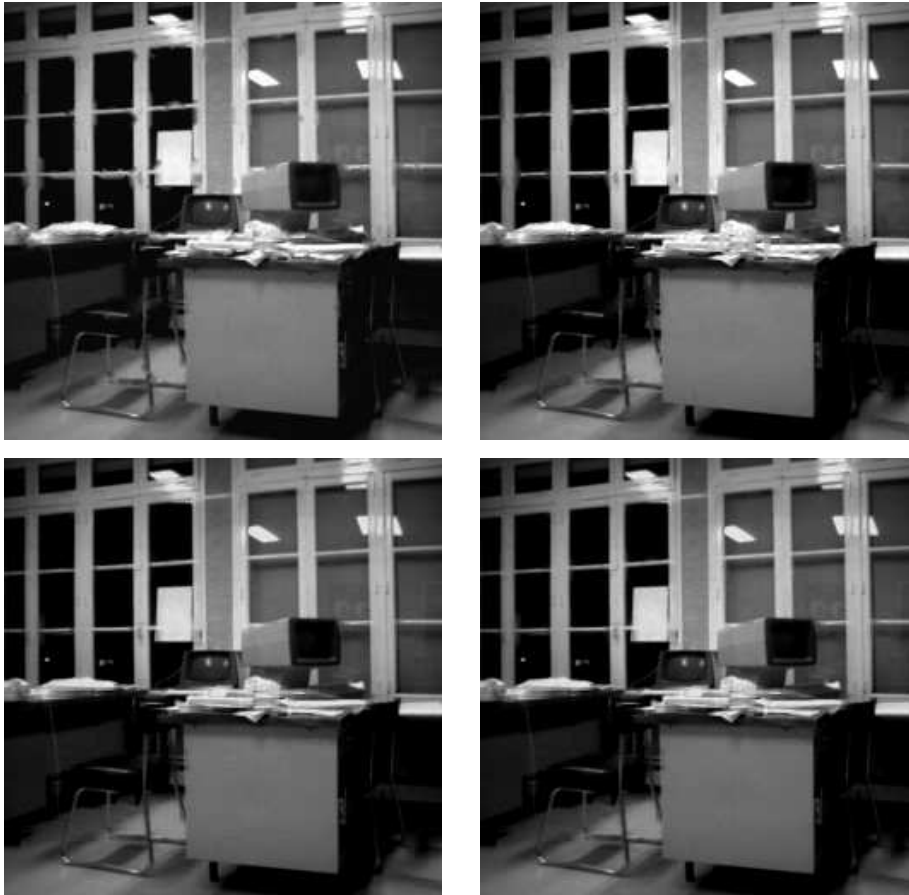
FIG. 5.3. Interpolation of the image in Fig. 5.2. Top left: cubic interpolation by the MATLAB procedure "griddata" ( PSNR=30.18 , err_2 = 7.89 , err_1 = 1.51 ). Top right: Algorithm (A), ( PSNR=31.61 , err_2 = 6.69 , err_1 = 1.36 ). Bottom left: Algorithm (B), ( PSNR=34.08 , err_2 = 5.03 , err_1 = 0.93 ). Bottom right: Algorithm (C), ( PSNR=33.98 , err_2 = 5.09 , err_1 = 0.97 ). The images at the top contain artifacts, in particular at the left window side. The algorithms at the bottom show a better performance and do not introduce these artifacts.
