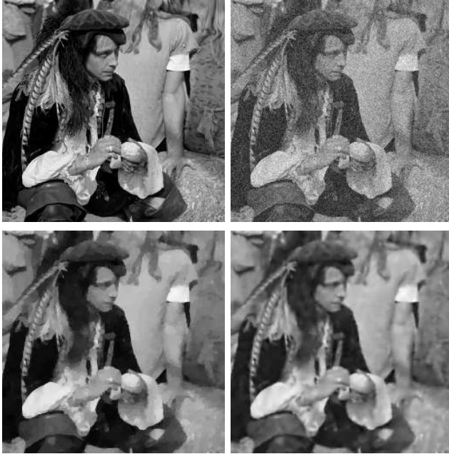
Fig. 2: Top: Original image of size 256 \times 256 with values in [0, 255] and noisy image (Gaussian noise with standard deviation 25). Bottom: Reconstruction via the Rudin-Osher-Fatemi model (21) and regularization parameter \lambda = 25 (left) and model (24) with \lambda = 15 (right).
