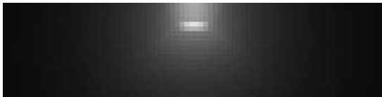
Figure 5.4: Here, a part of the image done with an edge geometry with distance 0.5\text{mm} is shown. The edge itself is along the upper border of the image. A bright spot is clearly visible near the center of the image.
