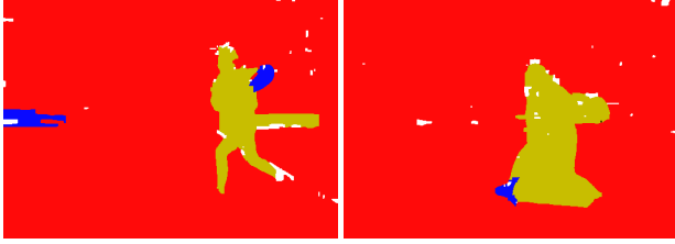
Figure 8. Segmentation by superpixel voting on the sample images shown in Fig. 7. Homogenous regions with few trajectories are dominated by false labels close to the object boundary.
