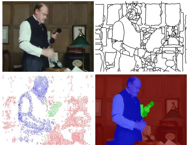
Figure 1. Object segmentation in videos based on point trajectories [7] yields sparse object labels. We propose a hierarchical variational model that propagates these labels preferably in homogenous regions. As a result we obtain a dense segmentation that reveals an even higher classification accuracy than the sparse labels and overcomes the over-segmentation issue of static image segmentation approaches [1].
