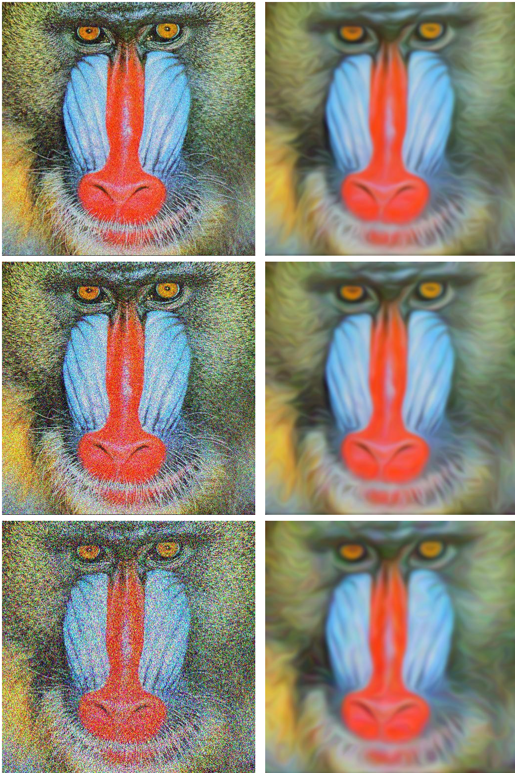
Figure 5.8: Left: baboon with additive Gaussian noise of variance (top to bottom) 30, 50, 100. Right: filtered with anisotropic diffusion using \varrho = 3 and autonomous decorrelation time T = 52, 61, 98 , respectively. The remaining parameters were set as in Figure 5.7.
