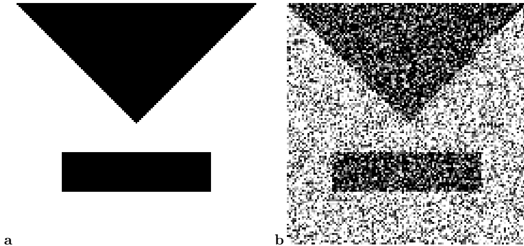
Figure 5.1: Ideal and noisy input image ( [0, 127]^2 \rightarrow [0, 255] ) for the ‘Triangle and rectangle’ experiment. Noise with uniform distribution in the range [-255, 255] was added to the two-valued synthetic data.
