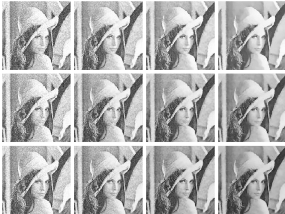
Figure: Comparison of different solvers. Top: Adaptive software preconditioned CG [sic!]. Middle: Jacobi solver on graphics hardware. Bottom: CG solver on graphics hardware. Authors: M. Rumpf and R. Strzodka.
