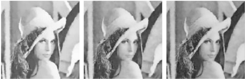
Figure: Comparison of different solvers (Zoom). Left: Adaptive software preconditioned CG [sic!]. Middle: Jacobi solver on graphics hardware. Right: CG solver on graphics hardware. Authors: M. Rumpf and R. Strzodka.
