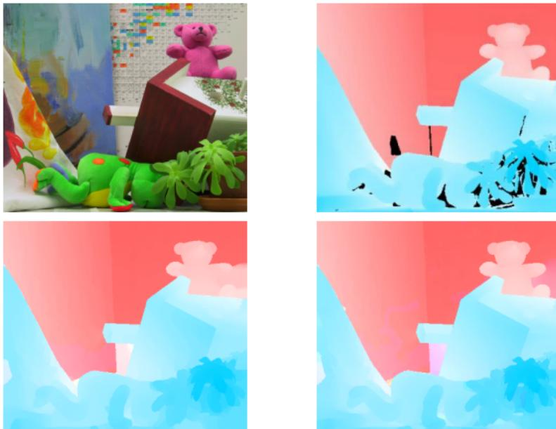
**Figure:** **top left:** first image frame **top right:** ground truth flow **bottom left:** result without nonlocal regularisation **bottom right:** result with nonlocal regularisation
