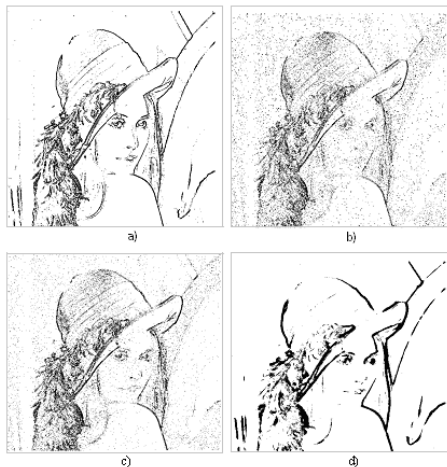
Figure: The 9-10% pixels with the highest evaluation according to the presented operators, a) Roberts, b) Laplace4, c) Laplace8, d) Gauß
