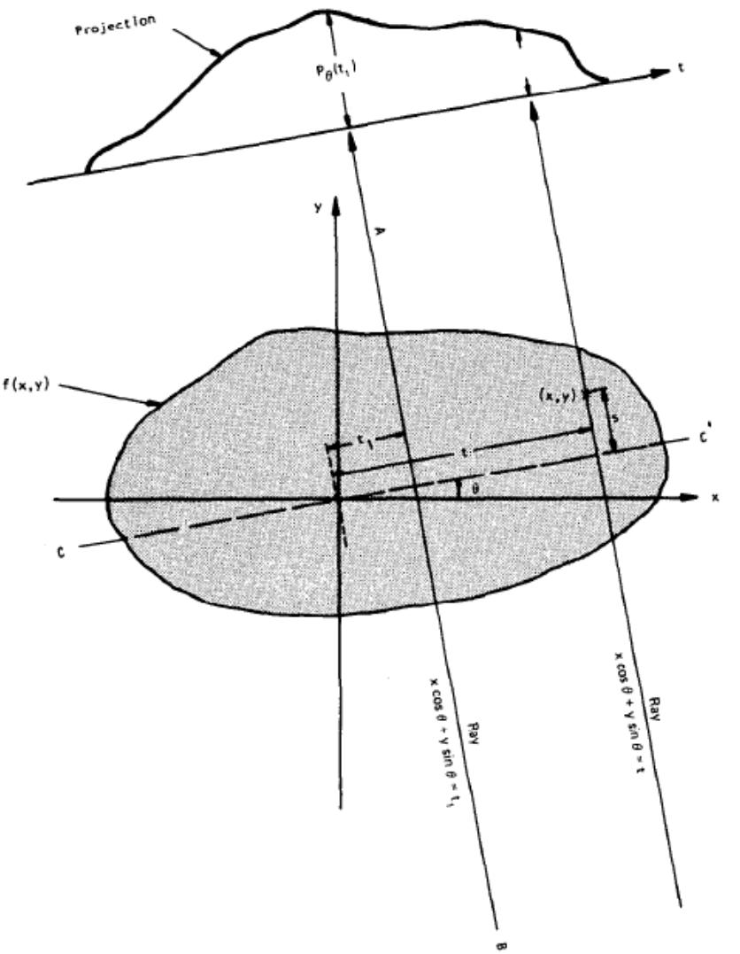
Figure 4: Object,  $f(x, y)$ , and its projection,  $P_\theta(t_1)$ , shown for angle  $\theta$ . Source: Kak, 1979.
