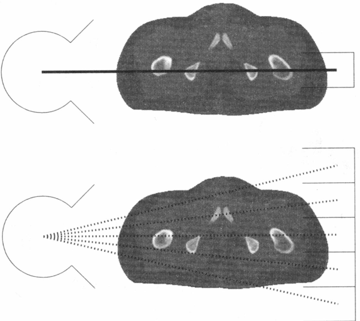
Figure 2: Dual motion scanner. **Top:** One source, one detector. **Bottom:** One source, several detectors. Source: Natterer & Wübbeling, 2001.
