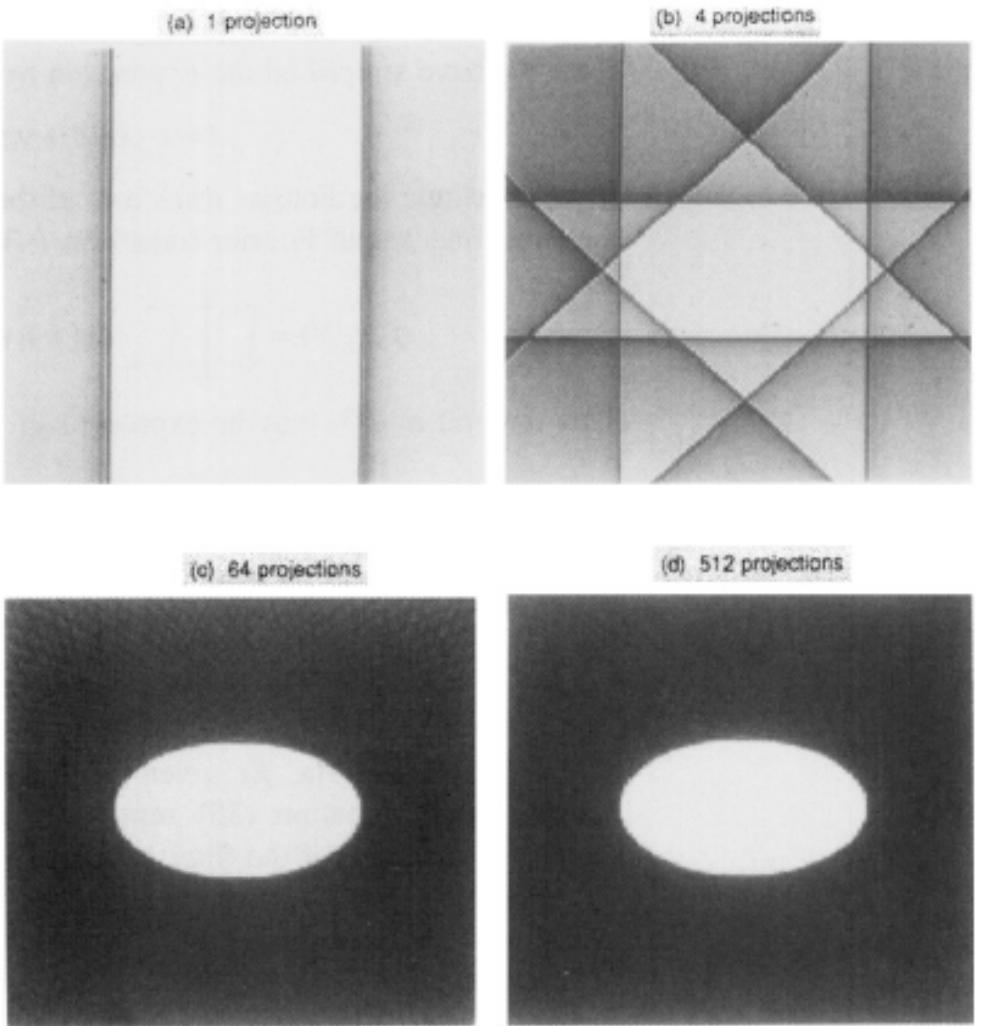
Figure 13: The result of backprojecting the projection of an ellipse. **(a)** shows the result of backprojecting for a single angle, **(b)** shows the effect of backprojecting over 4 angles, **(c)** shows 64 angles, and **(d)** shows 512 angles.
