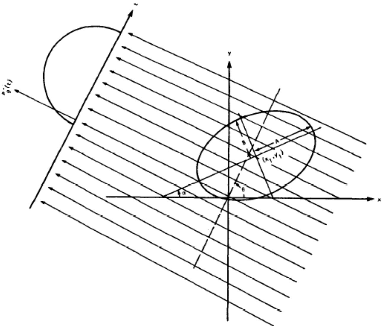
Figure 9: Analytical calculation for an ellipse with its center located at  $(x_1, y_1)$  and its major axis rotated by  $\alpha$ . Source: Rosenfeld & Kak, 1982.
