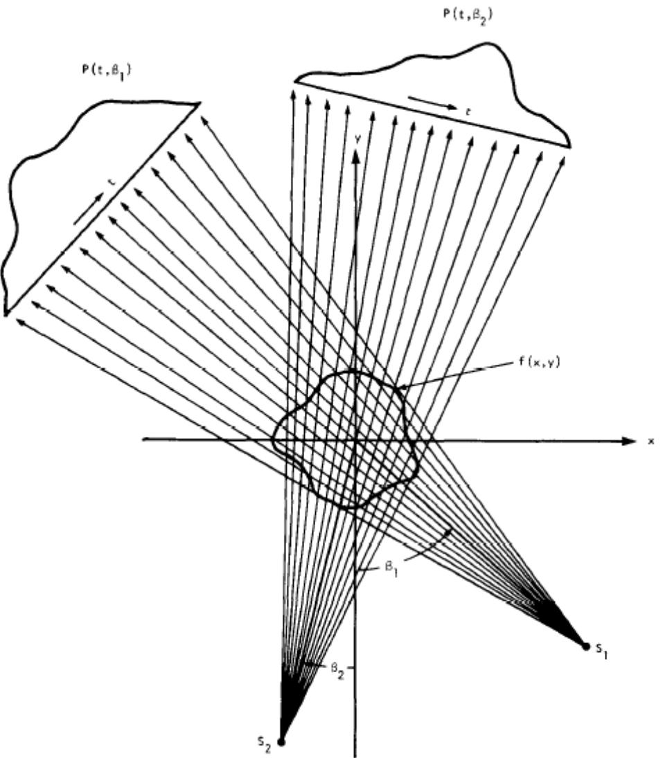
Figure 6: A fan beam projection is collected if all the rays meet in one location. Source: Rosenfeld & Kak, 1982.
