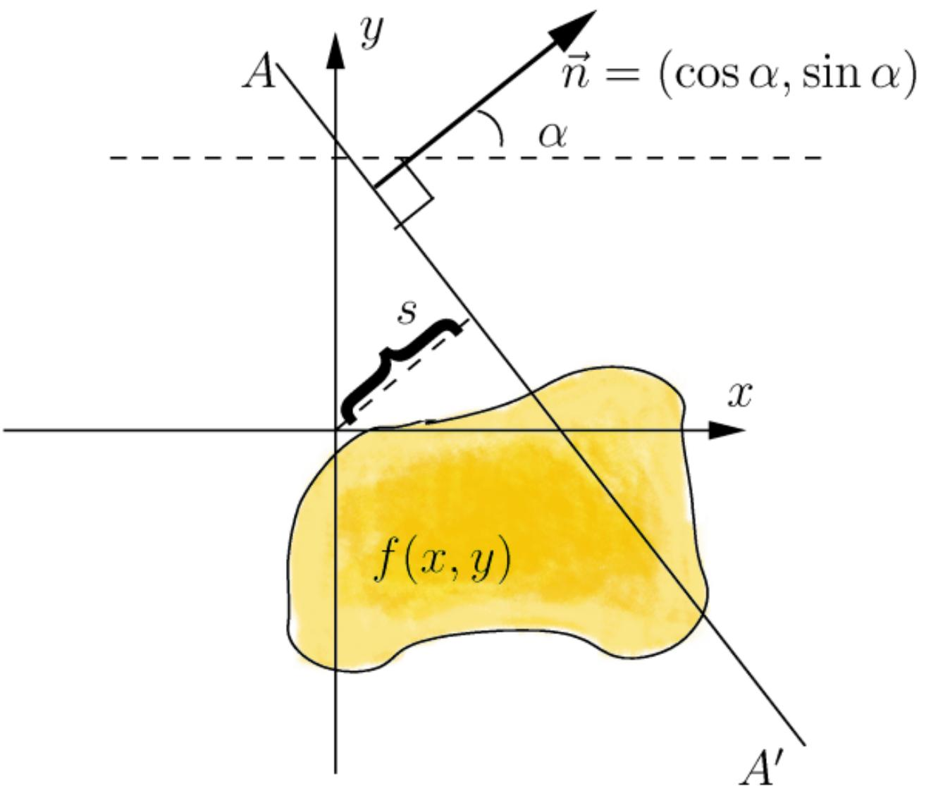
Figure 1: Radon Transform: Attenuation
