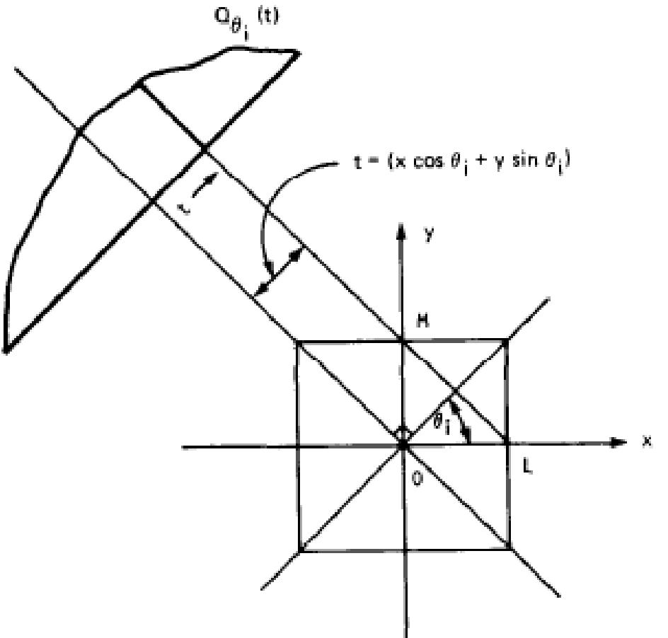
Figure 12: Reconstructions are often done using a procedure known as backprojection. Here a filtered projection is smeared back over the reconstruction plane along lines of constant  $t$ . The filtered projection at a point  $t$  makes the same contribution to all pixels along the line  $LM$  in the  $x - y$  plane.
