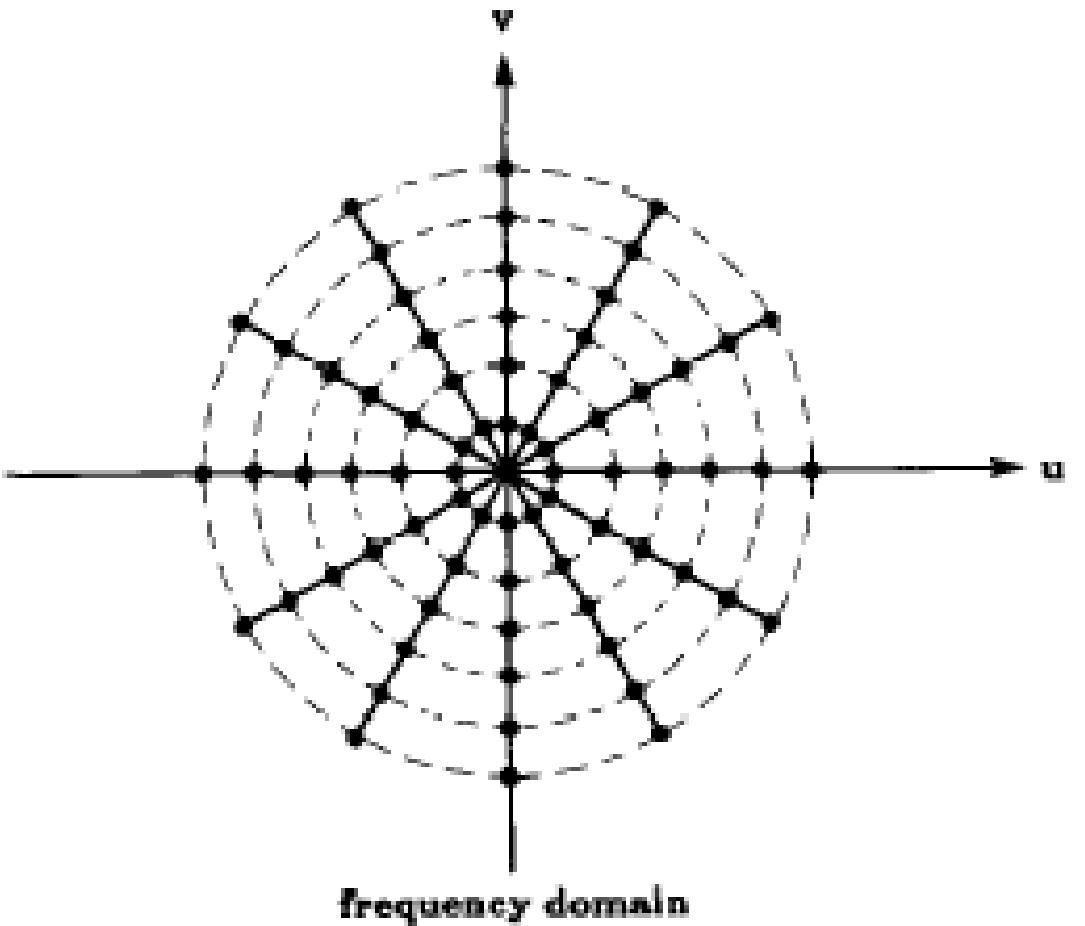
Figure 11: Collecting projections of the object at a number of angles gives estimates of the Fourier transform of the object along radial lines. The dots represent the actual location of estimates of the object's Fourier transform. Source: Pan & Kak, 1983.
