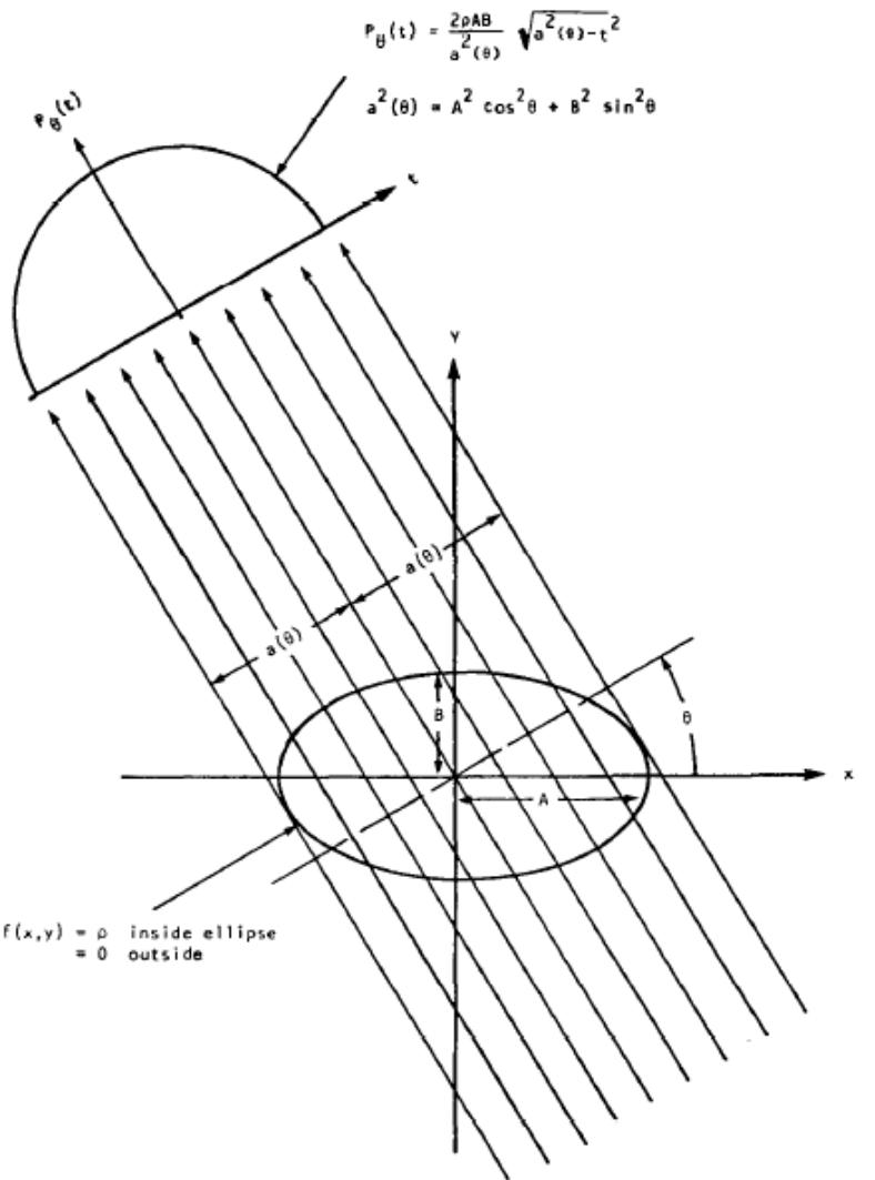
Figure 8: Analytic expression is shown for the projection of an ellipse. For computer simulations a projection can be generated by simply summing the projection of each individual ellipse. Source: Rosenfeld & Kak, 1982.
