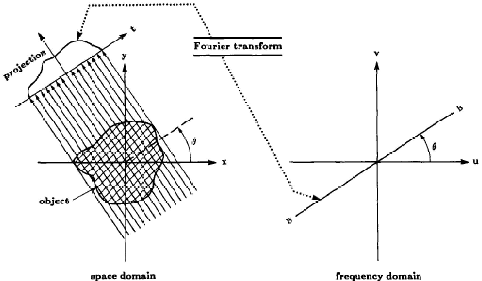
Figure 10: The Fourier Slice Theorem relates the Fourier transform of a projection to the Fourier transform of the object along a radial line. Source: Pan & Kak, 1983.
