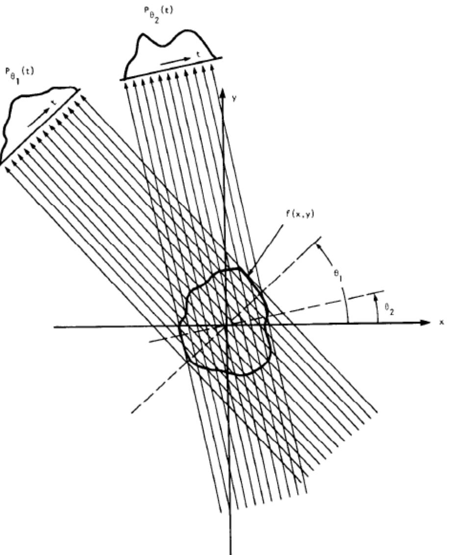
Figure 5: Parallel projections are taken by measuring a set of parallel rays for a number of different angles. Source: Rosenfeld & Kak, 1982.
