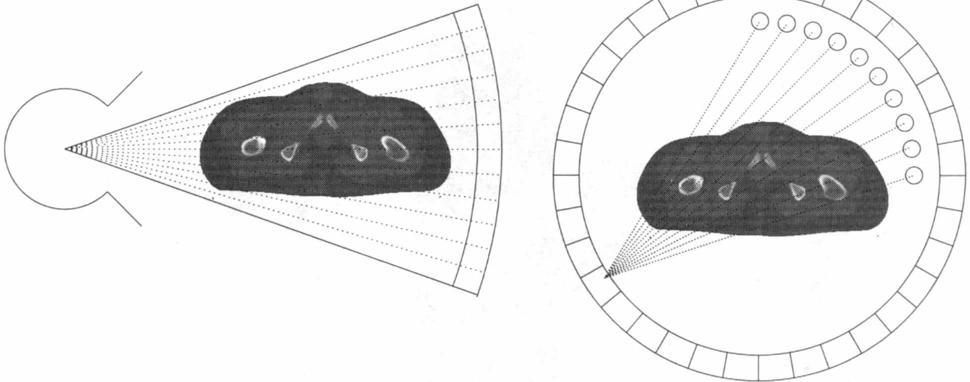
Figure 3: Fan beam scanning. **Left:** Rotating detector-source system. **Right:** Stationary detector ring, rotating source. Source: Natterer & Wübbeling, 2001.
