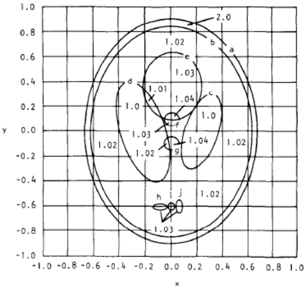
Figure 7: **Left:** The Shepp and Logan head phantom. **Right:** The phantom is a superposition of 10 ellipses. Source: Rosenfeld & Kak, 1982.
