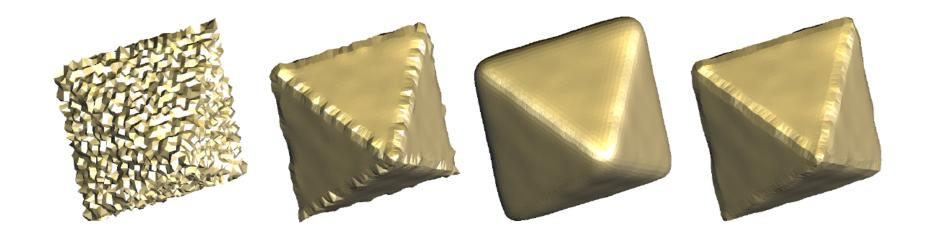
**Left to right:** A noisy octahedron surface, smoothed by isotropic nonlinear 3D diffusion (Perona-Malik model), mean-curvature motion, and anisotropic geometric diffusion (U. Clarenz, U. Diewald, M. Rumpf 2000)
