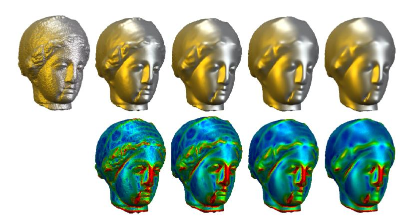
**Top left:** Noisy 3D scan image of a sculpture. **Top row, to right:** Filtered by anisotropic geometric diffusion, threshold  $\lambda=10$ , pre–smoothing  $\rho=0.02$ , at evolution times T=0.0002, T=0.0004, T=0.0006, T=0.0008. **Bottom:** Same filtered surfaces as above, with colour-coded principal curvatures (U. Clarenz, U. Diewald, M. Rumpf 2000)
