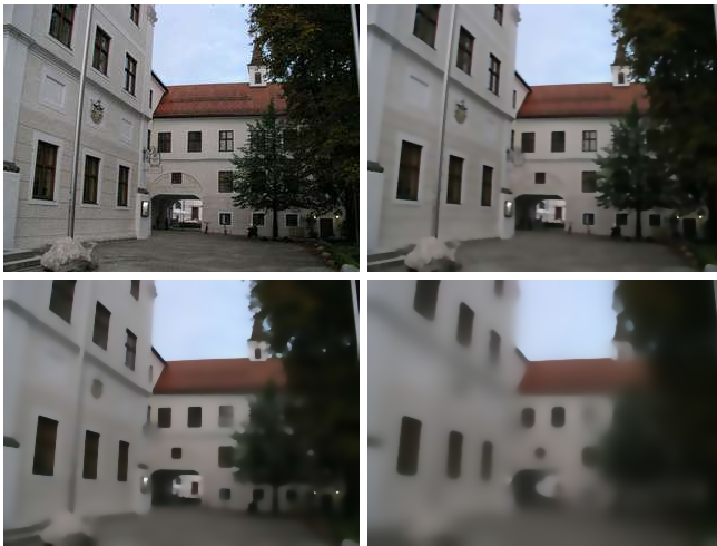
Figure: Original image (top left) smoothed by isotropic nonlinear diffusion, t = 2.5 , t = 10 , t = 40 .
