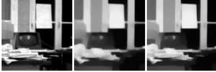
Fig. 1. Left: Original image, 93 \times 93 pixels. Middle: TV diffusion with standard explicit scheme, where TV diffusivity is regularised with \varepsilon = 0.01 , \tau = 0.0025 , 10000 iterations. Right: TV diffusion with 2 \times 2 -pixel scheme (20) without regularisation of diffusivity, \tau = 0.1 , 250 iterations.
