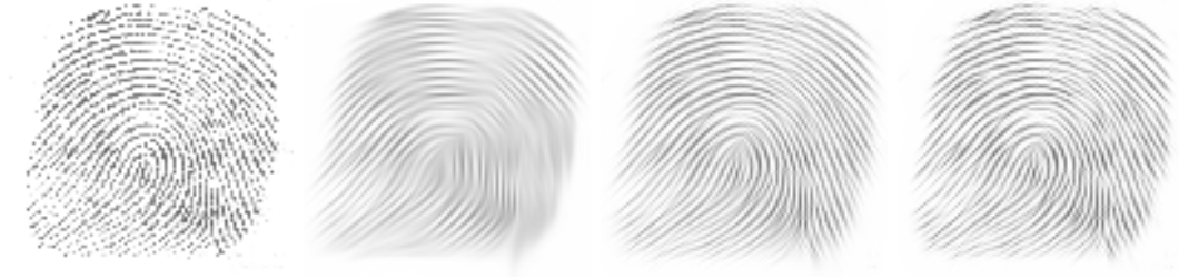
Figure 12: Left to right: (a) Fingerprint image, 100 \times 100 pixels. (b) Filtered with CED, \varepsilon = 0.001 , C = 1 , \sigma = 0.5 , \varrho = 4 , using the nonnegativity scheme [54] with \tau = 1/6 and N = 60 iterations. (c) Processed with our LSAS scheme ( \alpha = 0 ) for CED, same parameters. (d) LSAS scheme with \tau = 1 and N = 10 iterations.
