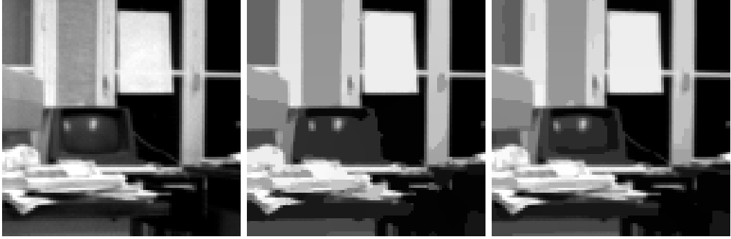
Figure 7: Left to right: (a) Original image from Figure 3, 93 \times 93 pixels. (b) Processed by nonlinear isotropic diffusion, contrast parameter \lambda = 3 , noise scale \sigma = 0.5 , with standard explicit scheme, time step size \tau = 0.25 , N = 1600 iterations. (c) Processed by nonlinear isotropic diffusion, same parameters as (b), with LSAS, \alpha = 0.5 , \tau = 0.25 , N = 1600 .
