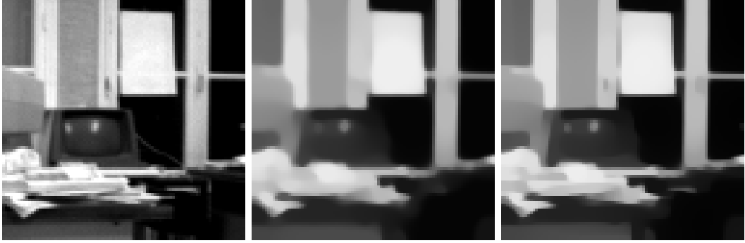
Figure 3: Left to right: (a) Original image, 93 \times 93 pixels. (b) TV diffusion with standard explicit scheme, where TV diffusivity is regularised with \varepsilon = 0.01 , \tau = 0.0025 , 10000 iterations. (c) TV diffusion computed with LAS without regularisation of diffusivity, \tau = 0.1 , 250 iterations.
