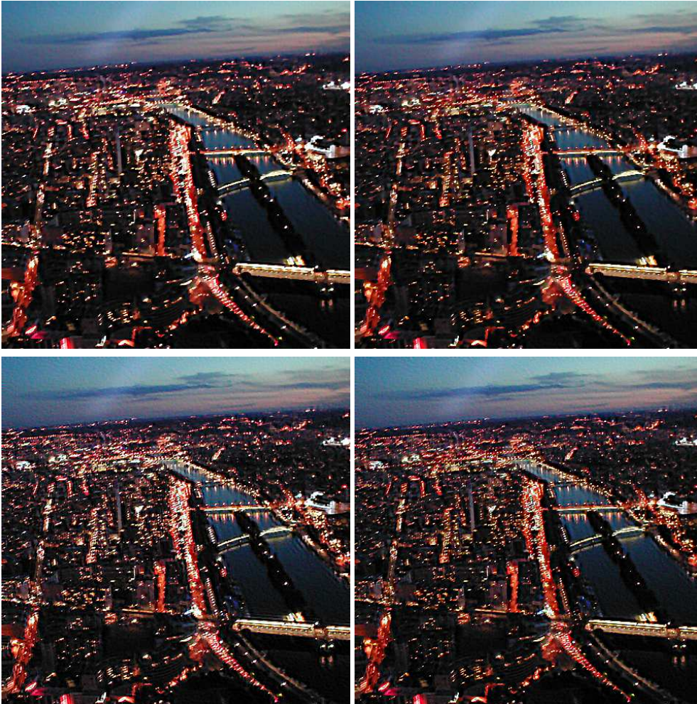
Figure 7.1: Variational deconvolution of the colour photograph from Figure 6.8(a), using the approximate space-invariant PSF from Figure 6.1(e). In all cases, robust L^1 data terms and Perona–Malik regularisers with \lambda = 26 have been used. In this setting, regularisation weights can be compared. Top left (a) : Without constraint, \alpha = 0.06 (same as Figure 6.8(d)). – Top right (b) : With positivity constraint, \alpha = 0.06 . – Bottom left (c) : Without constraint, \alpha = 0.03 . – Bottom right (d) : With positivity constraint, \alpha = 0.03 . – Following [220].
