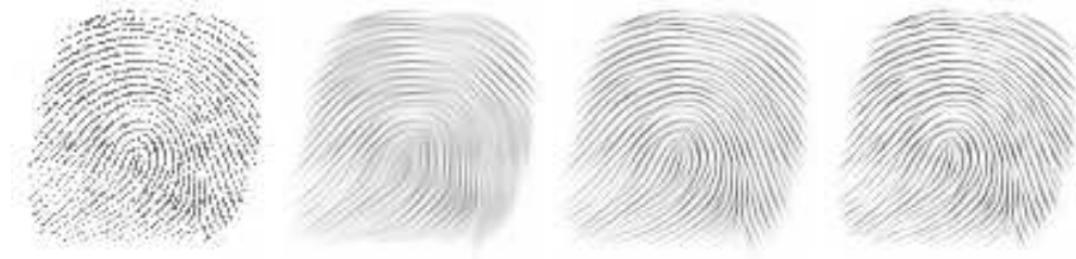
Figure 4.12: Left to right: (a) Fingerprint image, 100 \times 100 pixels. (b) Filtered with CED, \varepsilon = 0.001 , C = 1 , \sigma = 0.5 , \varrho = 4 , using the nonnegativity scheme [206] with \tau = 1/6 and N = 60 iterations. (c) Processed with our LSAS scheme ( \alpha = 0 ) for CED, same parameters. (d) LSAS scheme with \tau = 1 and N = 10 iterations.
