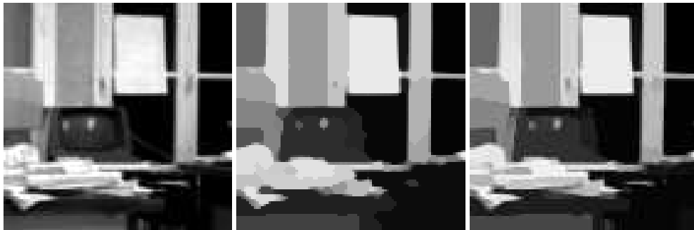
Figure 4.7: Left: Original image, 93 \times 93 pixels. Middle: Balanced forward-backward diffusion with standard explicit scheme, \varepsilon = 0.1 , \tau = 0.0025 , 160000 iterations. Right: BFB diffusion with our LAS, \tau = 0.1 , 4000 iterations.
