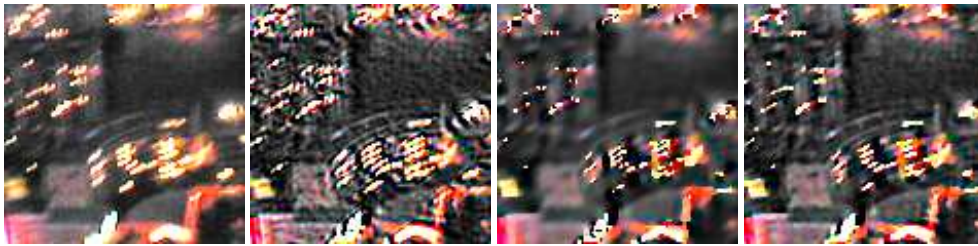
Figure 6.11: Enlarged detail views ( 117 \times 117 pixels) from the images shown in Figure 6.8, bottom left region, with linearly enhanced contrast. Left to right: (a) Original image. – (b) Quadratic data term, quadratic regulariser. – (c) Quadratic data term, Perona–Malik regulariser. – (d) Robust data term, Perona–Malik regulariser. – In this low-contrast region, the deconvolution result (b) is dominated by artifacts while in (c) the strong regularisation needed leads to a partial loss of details like the building contours. The reduced amount of regularisation with robust data terms (d) allows for a better preservation of these features. – Partially following [223].
