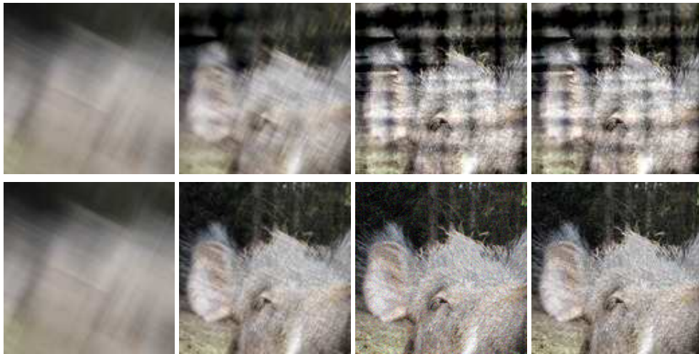
Figure 6.5: Deblurring of a detail of the Styrian Hog photograph from Figure 6.4 with different boundary treatment. Top, left to right: (a) Photograph detail blurred with discontinuous kernel from Figure 6.1(d). – (b) Linear deblurring by Wiener filter. – (c) Diffusion–reaction deblurring with TV diffusivity. – (d) Diffusion–reaction deblurring with Perona–Malik diffusivity. In (b)–(d), a continuous periodic extrapolation of the blurred image was used (realistic method). While details are well reconstructed, shadow-like boundary artifacts affect the overall quality. Bottom row (e)–(h): Same as (a)–(d) but with special setting to suppress boundary artifacts. The image was extended by reflection to four times its original size before blurring. This quadruple-size blurred image was then blurred and deblurred with periodic continuation. – Images: D. Theis, from [222].
