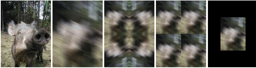
Figure 6.2: Left to right: (a) Styrian Hog photograph, 240 \times 320 pixels. – (b) Blurred with linear motion blur (40 pixels horizontal, 20 pixels vertical, compare Figure 6.1(c)). (a) and (b) were clipped from a larger image, such that the information transport across the boundary is correctly simulated. – (c) Blurred image extended by mirroring, corresponding to reflecting boundary conditions. The blur assumption is severely violated in the amended regions. No discontinuities are introduced. – (d) Periodic image extension. The blur assumption is fulfilled in the interior of the amended regions. It is violated at the boundaries themselves, where also discontinuities are introduced. – (e) Zero-padding extension. Violation of blur assumptions and introduction of discontinuities are analog to (d). – Images (c), (d): D. Theis.
