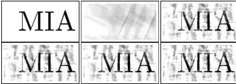
Figure 6.6: Top left (a) : Grey-value MIA Letters test image. Top middle (b) : Blurred with discontinuous kernel from Figure 6.1(d). Top right (c) : Linear deblurring by Wiener filter, boundary treatment by continuous extrapolation. Bottom left (d) : Diffusion-reaction deblurring with TV diffusivity and continuation strategy (2 levels). Bottom middle (e) : Same with Perona–Malik diffusivity. Bottom right (f) : Same with anisotropic diffusion tensor. – From [222]. Deconvolved images: D. Theis.
