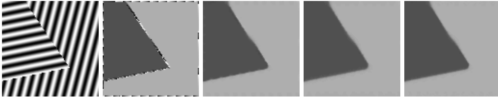
Figure 3.10: Left to right: (a) Synthetic image with oriented textures, inspired by [199]. (b) Local orientations computed via derivatives of Gaussians. Orientations have been mapped to grey-values. Note that the orientations represented by black and white are close neighbours. (c) Orientations after median filtering of the orientation matrices with Frobenius norm and a disk-shaped structure element of diameter 7. (d) Same with structure element of diameter 9. (e) Spectral norm median filtering, diameter 9. Image: F. Becker, from [217].
