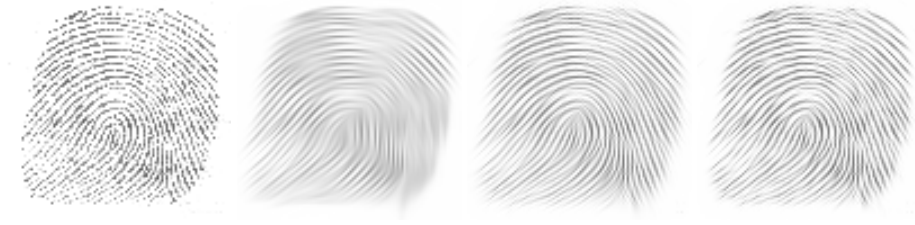
Fig. 5. Left to right: (a) Fingerprint image, 100 \times 100 pixels. (b) Filtered with the nonnegativity scheme [25] for CED with C = 1 , \sigma = 0.5 , \varrho = 4 , \tau = 1/6 , and N = 60 iterations. (c) Processed with our LSAS algorithm for CED, same parameters. (d) LSAS algorithm with \tau = 1 and N = 10 iterations.
