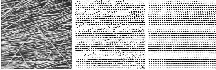
**Fig. 1. Left to right: (a)** Image containing oriented texture with inhomogeneities. **(b)** Structure tensors computed by smoothing the outer products  $\nabla u \nabla u^\top$  with  $15 \times 15$  Gaussian. The gradients themselves have been calculated by  $3 \times 3$  derivative-of-Gaussian filtering. The final matrix field has been subsampled for visualisation. **(c)** Result of median filtering of (b) with  $7 \times 7$  structure element and Frobenius norm (subsampled).
