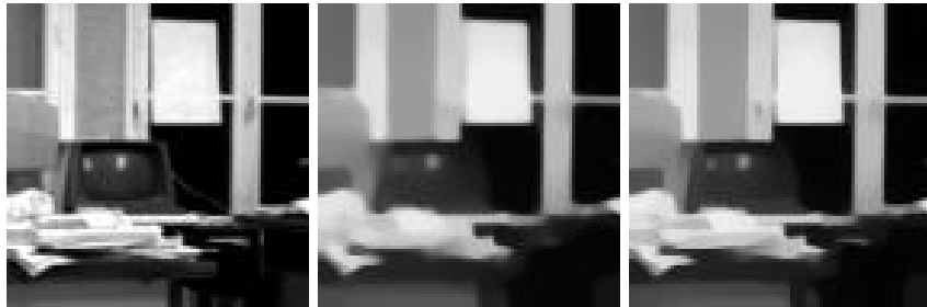
FIGURE 3. (a) Left: Original image, 93 \times 93 pixels. (b) Middle: Standard explicit scheme for regularised TV diffusion ( \varepsilon = 0.01 , \tau = 0.0025 , 10000 iterations). (c) Right: Same with four-pixel scheme without regularisation ( \tau = 0.1 , 250 iterations). Note that 40 times larger time steps are used. From [22].
