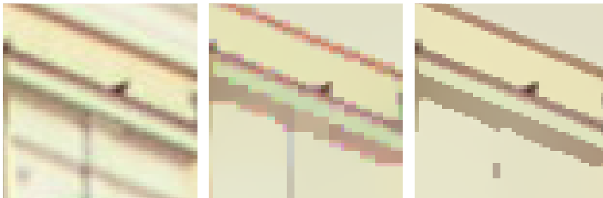
FIGURE 8. (a) Left: Zoom into an original image. (b) Middle: After classical wavelet shrinkage without coupling the RGB channels. (c) Right: Wavelet shrinkage with diffusion-inspired channel coupling.
