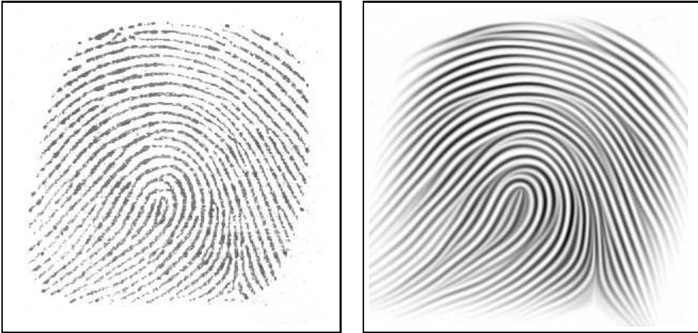
Figure 7: Test setting for nonlinear anisotropic coherence-enhancing diffusion filtering. (a) Left: Original fingerprint image ( 300 \times 300 pixels). (b) Right: Filtered reference image ( T = 256 , \sigma = 0.5 , \rho = 4 , \tau = 10^{-2} ), rescaled to [0, 255] .
