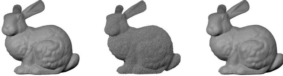
Figure 14: Test setting for anisotropic range image integration. (a) Left: One rendered image of Stanford Bunny . (b) Middle: Noisy range surface. (c) Right: Reconstruction computed with Fast Jacobi ( \omega_{\max} = 0.3 , n = 50 , 10 cycles).
