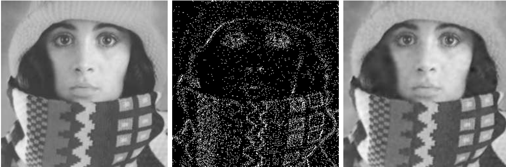
Figure 9: Biharmonic inpainting. (a) Left: Original image ( 256 \times 256 ). (b) Middle: Inpainting mask. (c) Right: Reconstruction with biharmonic inpainting in the unspecified regions (stopping time T = 10^6 ).
