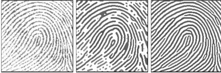
Fig. 1. Comparison between conventional and coherence-enhancing shock filtering. (a) Left: Fingerprint image, 186 \times 186 pixels. (b) Middle: Stationary state using the shock filter (5) with \sigma = 1.5 . (c) Right: Stationary state using coherence-enhancing shock filtering with \sigma = 1.5 and \rho = 5 .
