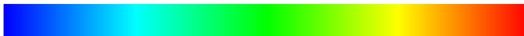
Figure 4.6: Colour code for reconstruction errors. Values of blue, green, and red denote locations in front, on, and behind the ground truth surface, respectively.
