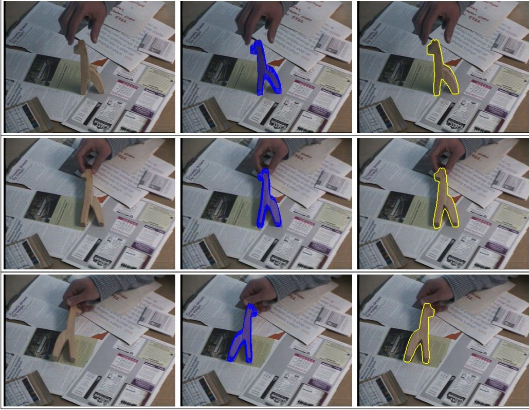
Figure 8: From left to right: Input image, estimated pose and extracted contour for three frames of a color sequence with a wooden giraffe. Top: Frame 32. Middle: Frame 64. Bottom: Frame 84. The surface model consists of a single closed point grid. Thus, it is possible to look through the projected pose. Note that this is irrelevant for contour-based pose estimation, where only silhouette points are needed.
