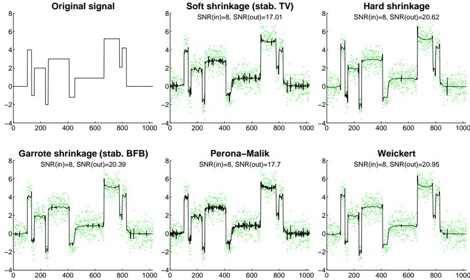
**Fig. 3.** Example of multiscale translation-invariant Haar wavelet denoising. Normal noise of  $\text{SNR}=8$  was added to the ideal signal, and different shrinkage functions have been applied. The noisy signal is represented by dots, reconstructed signal by solid line.
