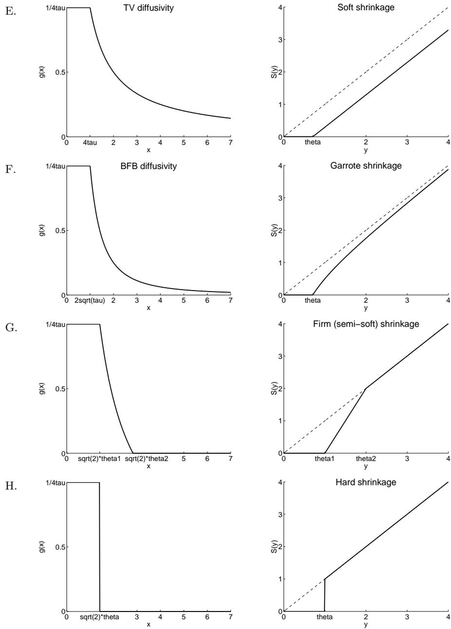
**Fig. 2.** Diffusivity functions (left), corresponding shrinkage functions (right). E. TV flow and soft shrinkage. F. Balanced forward-backward (BFB) diffusivity and garrote shrinkage. G. Firm shrinkage. H. Hard shrinkage. The functions are plotted for  $\tau = 0.25$  (which corresponds to  $\theta = \tau 2\sqrt{2}$  for soft shrinkage, and to  $\theta = \sqrt{2}\tau$  for garrote; the other use  $\theta = \theta_1 = 1, \theta_2 = 2$ ).
