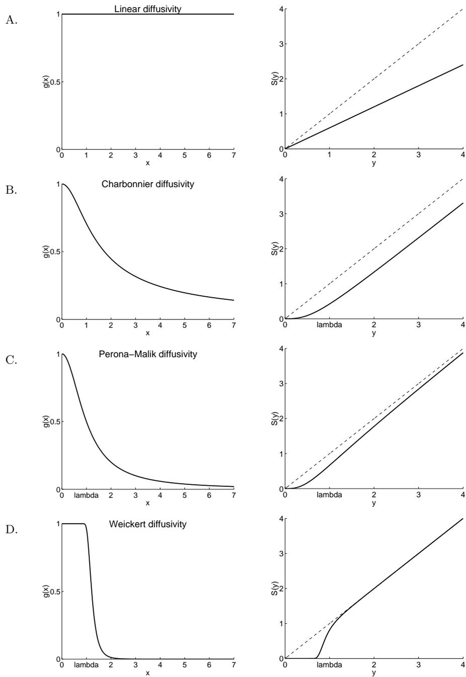
**Fig. 1.** Diffusivity functions (left), corresponding shrinkage functions (right).
