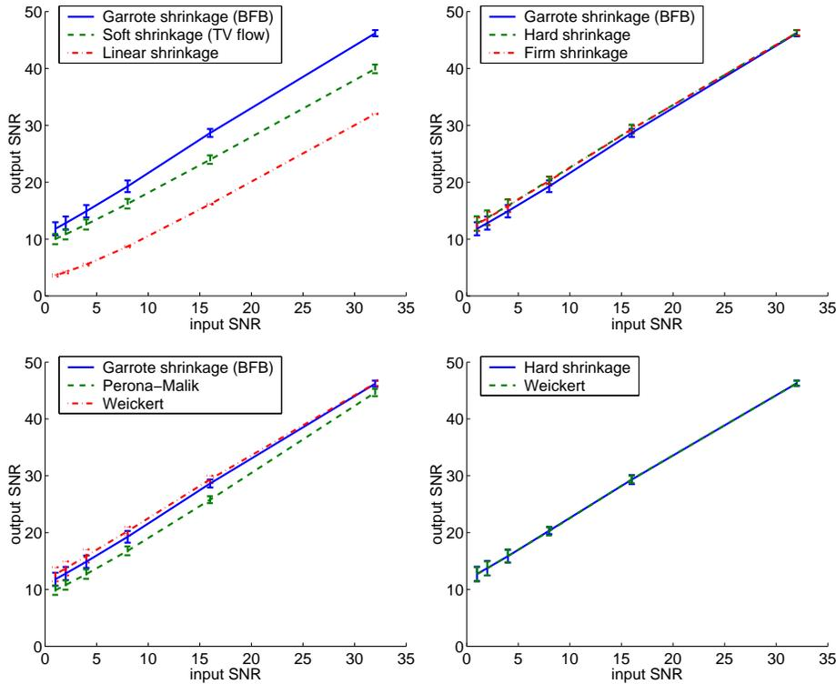
**Fig. 4.** Comparing the optimal denoising performance of shift-invariant multi-scale wavelet shrinkage with various shrinkage functions. SNR of the filtered signal is plotted against SNR of the input; the higher the graph, the better the result. The input signal was *blocks*, length 1024.
