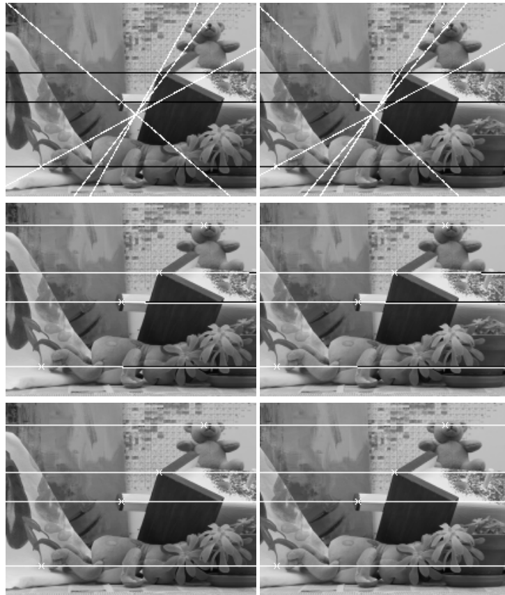
Fig. 1. Top Row: Left and right frame of the Teddy stereo pair (size 450 \times 375 ) with epipolar lines shown for the SIFT method (white) and the ground truth (black). Center Row: Ditto for the RANSAC-SIFT method (white) and the ground truth (black). Bottom Row: Ditto for the BBPW method (white) and the ground truth (black). Parameters have been optimised for \Delta F_{\text{truth}} .
