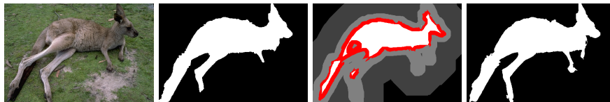
Fig. 6. Iterating the framework. From left to right: (a) Input kangaroo image. (b) Initial segmentation (error 7.2%). (c) User input. White depicts original user input, red visualises the updated input after the first iteration. (d) Final segmentation after second iteration (error 3.9%).
