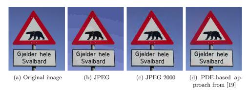
Figure 1.3: Comparison of lossy image compression methods: All images had a compression rate of 0.16 bits per pixel. Both JPEG and its successor JPEG 2000 contain visual artefacts whereas the the PDE-based reconstruction is almost flawless. Source: [19]
