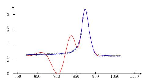
Figure 1.4: Interpolation of the popular titanium heat data (grey circles) [30] at the twelve locations marked by solid grey discs: The blue and red curve correspond to two cubic B-splines with different knot choices. Both splines interpolate the data at the same positions. The blue spline is considerably closer to the original data than the red spline.
