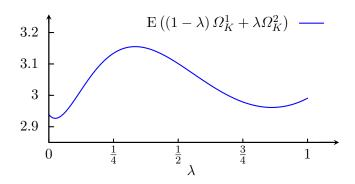
Figure 4.2: Evolution of the interpolation error with a linear spline for the function  $\exp(x)$  with mask points along the segment with endpoints  $\Omega_K^1 = \{-15, 10.65, 14.65, 15\}$  and  $\Omega_K^2 = \{-15, -1.2, 12.5, 15\}$ . It clearly depicts a non-convex behaviour. Note that the function values have been rescaled by a factor  $10^{-6}$  for better readability.
