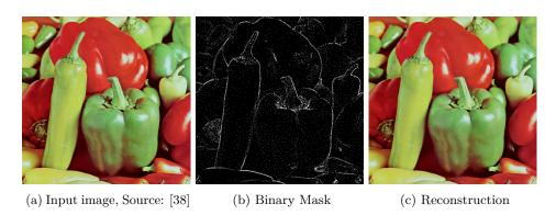
Figure 5.4: Test image Peppers in colour (511  $\times$  511): The reconstruction is done with an additional GVO on the binarised mask and presents a remarkable quality.
