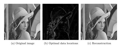
Figure 1.5: By optimally choosing 5% of the pixels from (a) we obtain the result in (c) by solving Eq. (1.1). The selected pixels are marked in white in (b). A Method to find the pixels in (b) is analysed in the forthcoming chapters. Source of the input image: [38]
