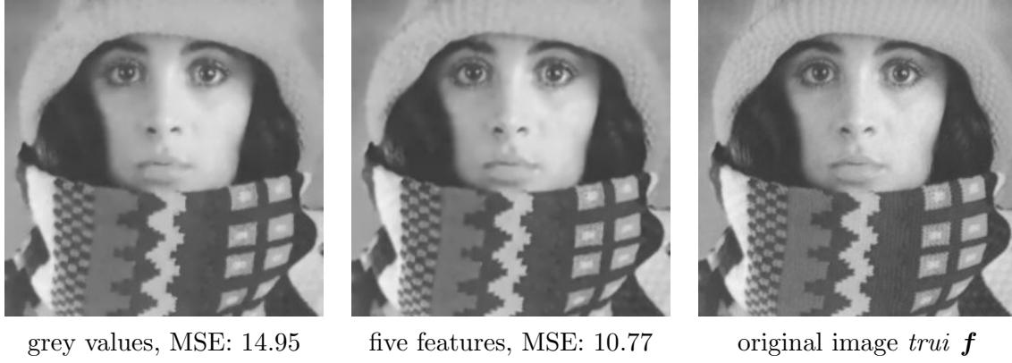
FIGURE 2.2: Illustration of EED inpainting using only grey-value features versus five features (grey values, \partial_x , \partial_y , 3 \times 3 and 5 \times 5 binomial kernels). The total mask density is 5% in both cases. The reconstruction error improves by nearly 28% compared to the already strong performance of classical EED inpainting.
