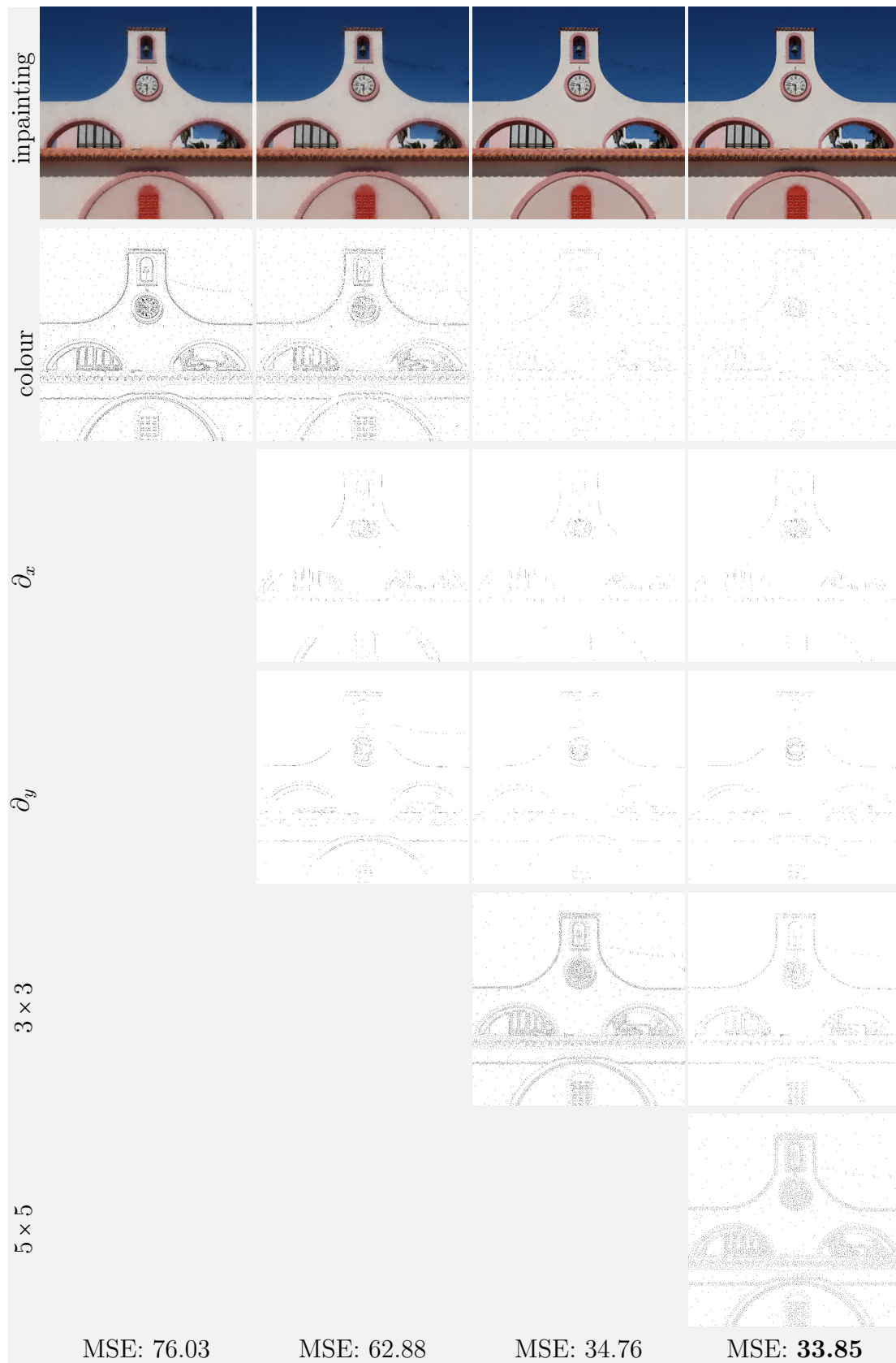
FIGURE 4.6: Harmonic inpainting results for a combined total mask density of 3% for elpaso produced with 30 densification iterations.
