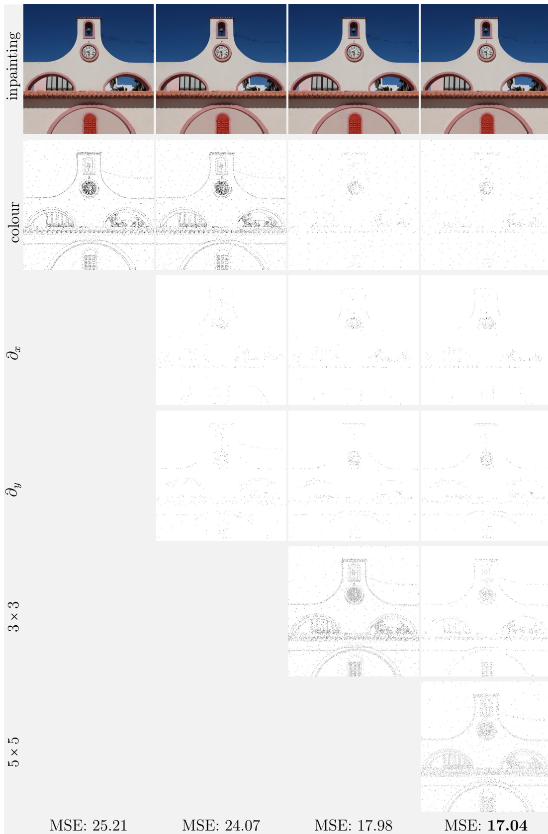
FIGURE 4.8: EED inpainting results for a combined total mask density of 3% for elpaso produced with 30 densification iterations
