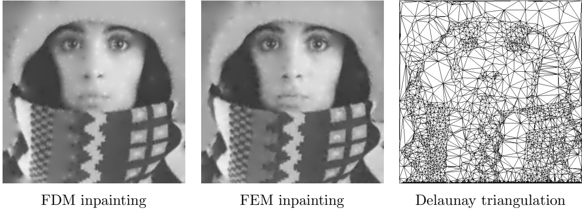
FIGURE 3.1: Harmonic inpainting with FDM and FEM. Note the logarithmic singularity suppression. Right: Delaunay triangulation used as the FEM mesh.
