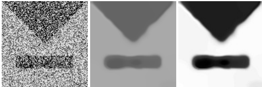
Fig. 2. (a) Left: Noisy test image, 128 \times 128 pixels. (b) Middle: After processing with the robustified bilateral process (36) with \sigma = 2 , \rho = 5 , \lambda = 1.4 , and t = 500 . (c) Right: After rescaling the filtered result from (b) to the greyscale interval [0, 255] .
