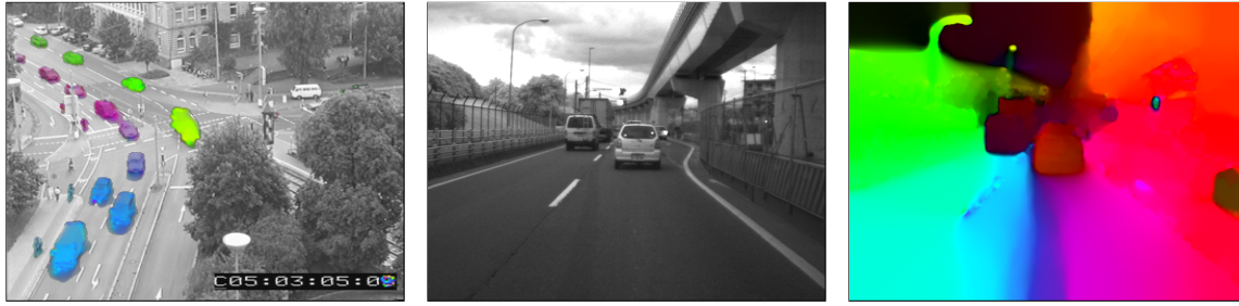
Fig. 1.2: Possible fields of application. Left: Tracking of cars in a traffic scene. Centre: Navigation of a car through a street. Right: Computed optic flow field. The colour indicates the direction of the relative motion.
