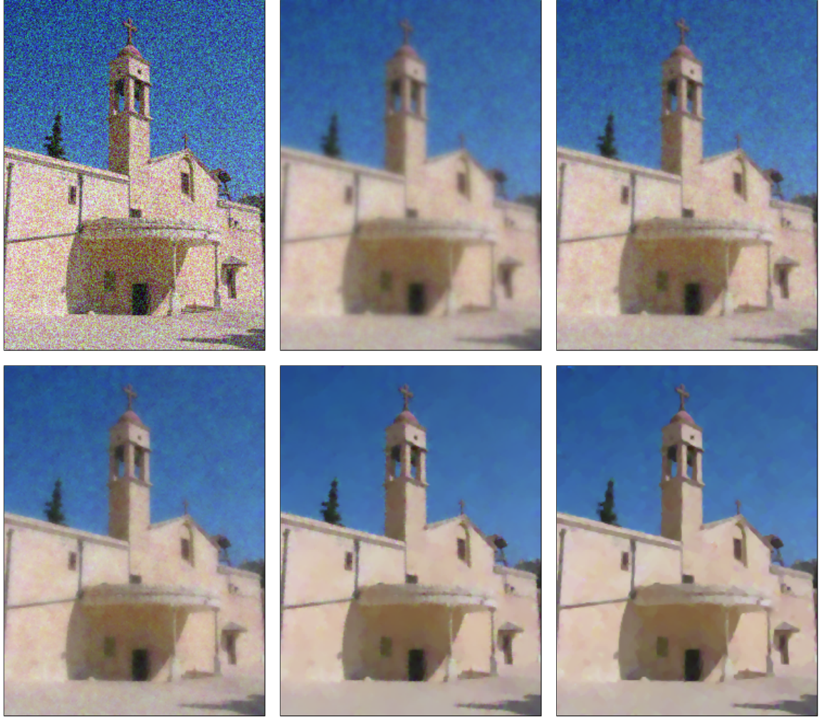
Fig. 2.11: Diffusion filtering of colour images. (a) Top Left: Noisy colour image. (b) Top Centre: Homogeneous diffusion. (c) Top Right: Linear isotropic diffusion. (d) Bottom Left: Linear anisotropic diffusion. (e) Bottom Centre: Nonlinear isotropic diffusion. (f) Bottom Right: Non-linear anisotropic diffusion.
