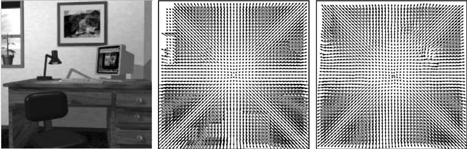
**Fig. 2.** (a) Left: Frame 10 of the *office* sequence. (b) Center: Ground truth flow field between frame 10 and 11. (c) Right: Computed flow field by our full multigrid CLG method ( $\sigma = 0.72$ ,  $\rho = 1.8$ , and  $\alpha = 2700$ ).
