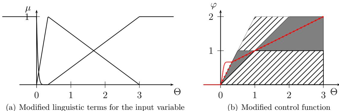
Figure 14: **Sine wave test.** Modified linguistic terms and modified control function of the improved MC scheme.
