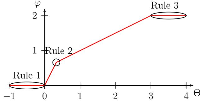
Figure 11: MC flux limiter
