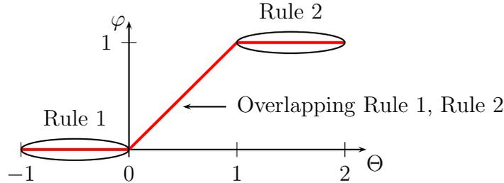
Figure 7: Control function of the Minmod scheme.
