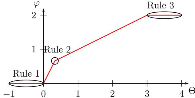
Figure 11: MC flux limiter
