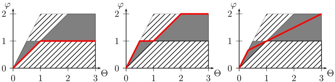
Figure 2: Flux limiters (strong line) and the Sweby TVD region (shaded). **Left.** Minmod limiter. **Middle.** Superbee limiter. **Right.** MC limiter.
