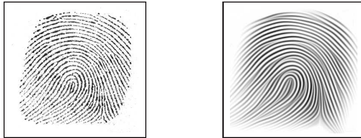
Fig. 2: Test image and reference image computed by a semi-implicit scheme. Left: Original image (finger, 300 \times 300 , rescaled to [0,255] for better visualisation). Right: CED-filtered reference image ( T = 300 , \lambda = 1 , \sigma = 0.5 , \rho = 4 , \alpha = 0.001 , \tau = 0.1 ), rescaled to [0,255]
