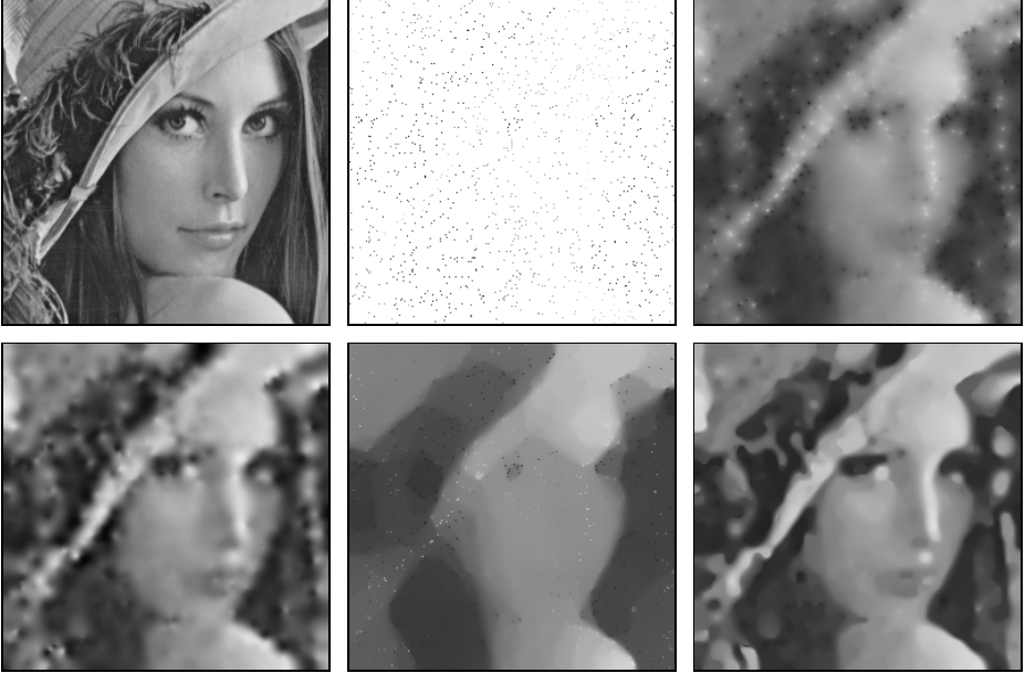
Fig. 1. (a) Top left: Zoom into the test image lena , 256 \times 256 pixels. (b) Top middle: Grey values of the scattered interpolation points (2 percent of all pixels, chosen randomly). (c) Top right: Interpolation by linear diffusion. (d) Bottom left: Biharmonic smoothing. (e) Bottom middle: Nonlinear isotropic diffusion ( \lambda = 0.1 ). (f) Bottom right: EED ( \lambda = 0.1 , \sigma = 1 ).
